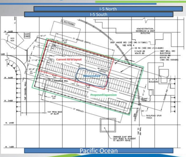
The existing ISFSI storage facility must be increased to accommodate approximately 100 additional canisters
