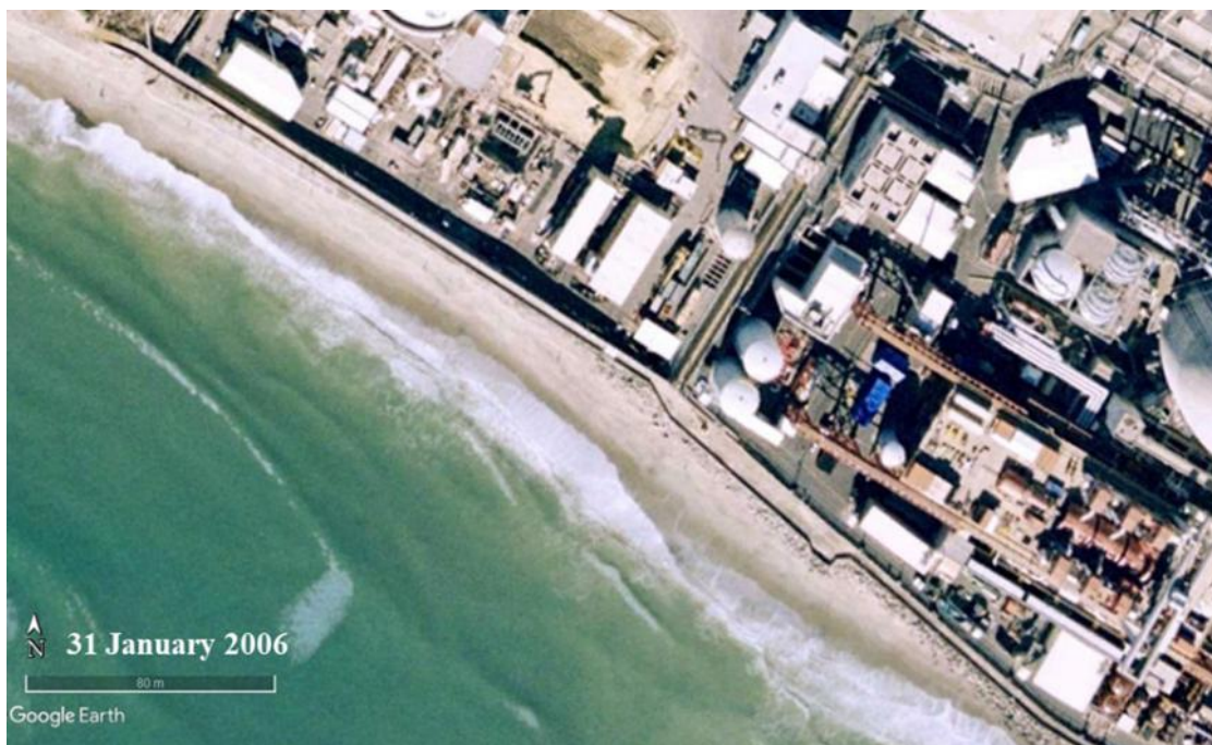
Photo C-7. Photograph showing revetment covered by sand and fronted by a wide beach at the northern end of SONGS (31 January 2006).
