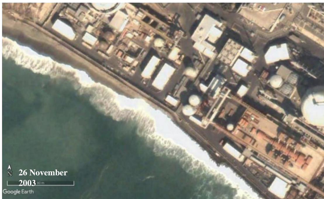
Photo C-3. Photograph showing waves attacking the revetment and the presence of a sand beach at the northern end of SONGS (26 November 2003).
