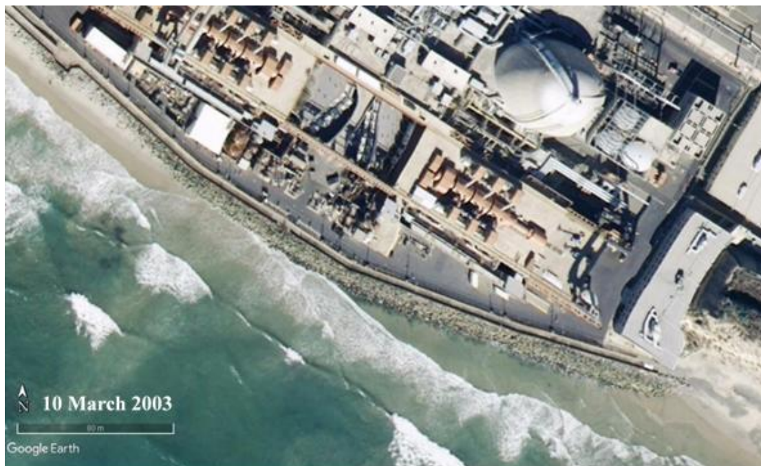
Photo C-2. Photograph showing waves from north swell attacking SONGS revetment at the southern end of SONGS (10 March 2003).
