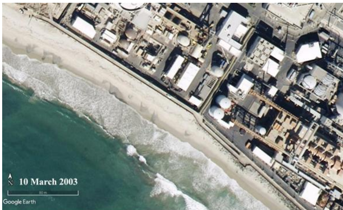
Photo C-1. Photograph showing revetment covered by sand and fronted by a wide beach at the northern end of SONGS (10 March 2003).
