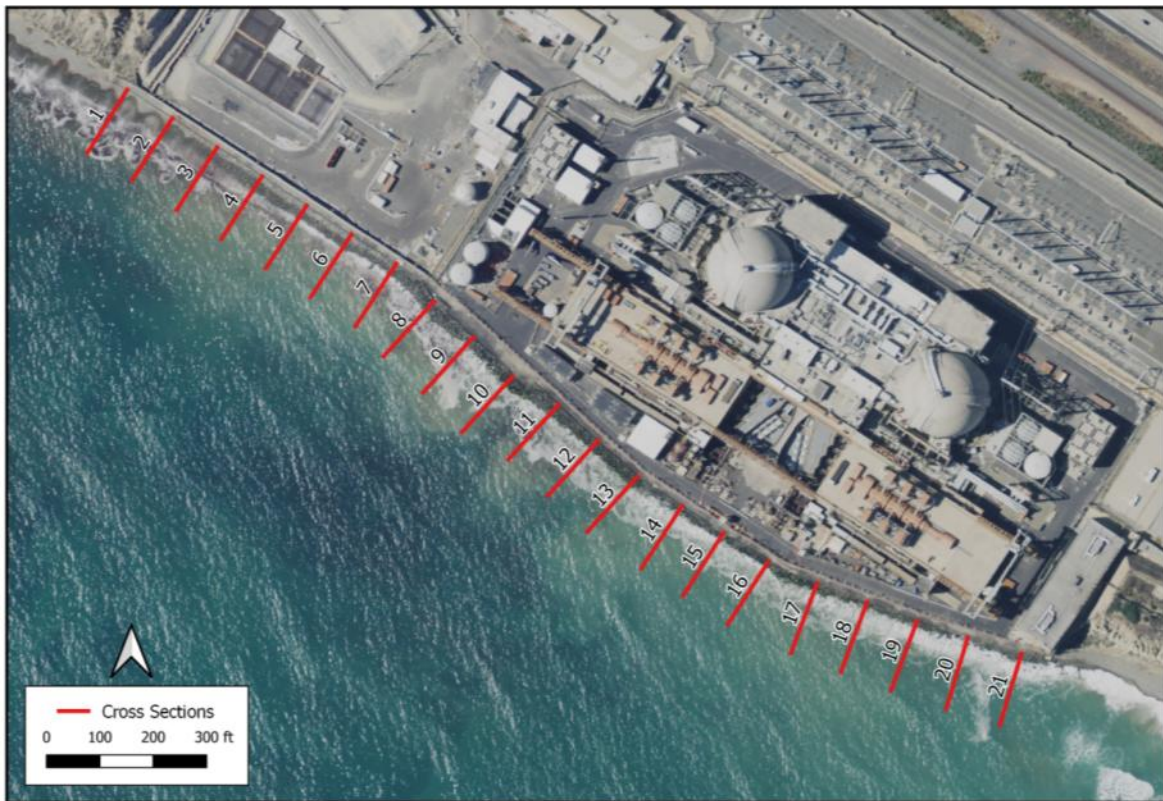
Figure 3-9. Location of 21 transects along the revetment, spaced 100 ft apart.
