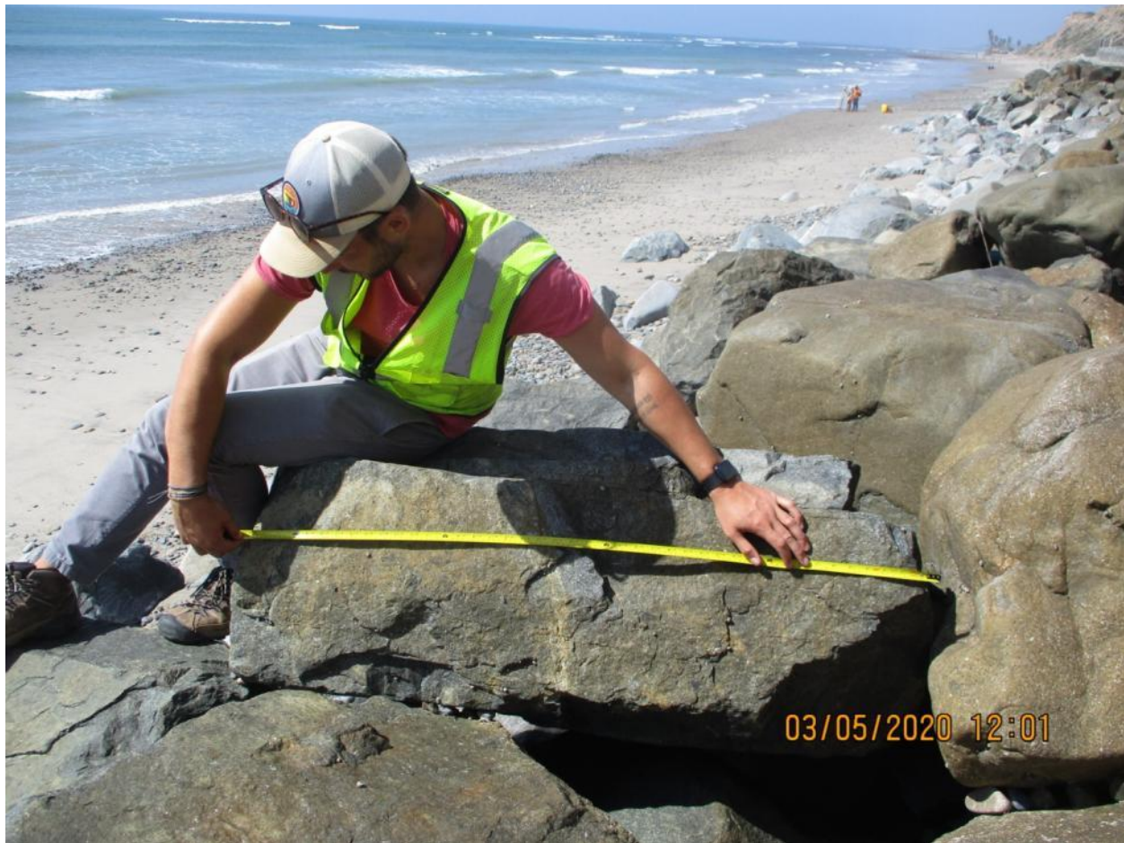
Figure 3-5. Measurements of the long axis of the rock (length).
