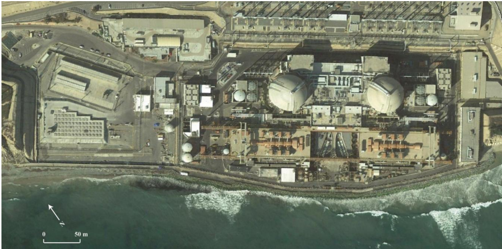
Figure 3-1. Photograph taken on 20 August 2018, showing the SONGS revetment. Notice the north part of the revetment is covered by beach sand.
