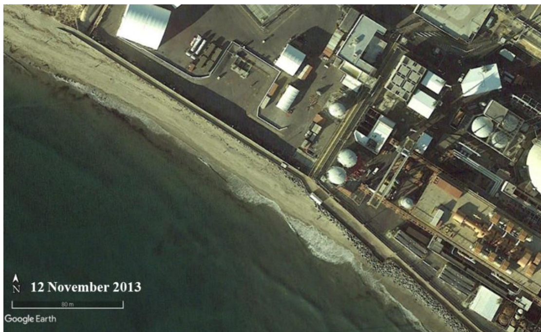
Photo C-11. Photograph showing revetment covered by sand and fronted by a wide beach at the northern end of SONGS (12 November 2013).
