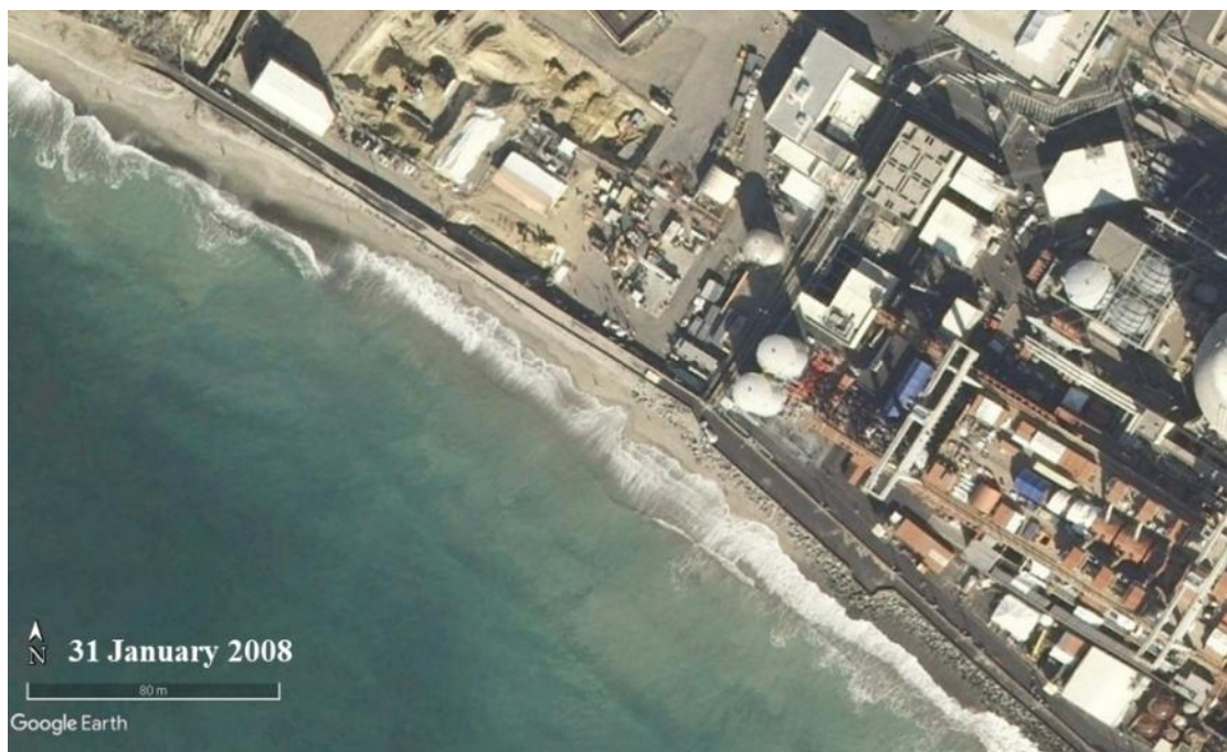
Photo C-9. Photograph showing revetment covered by sand and fronted by a wide beach at the northern end of SONGS (31 January 2008).
