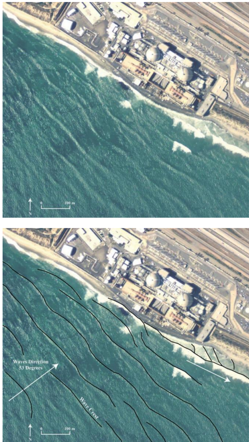
Figure 3-20. Waves attacking SONGS revetment at an angle and transporting sand south.
