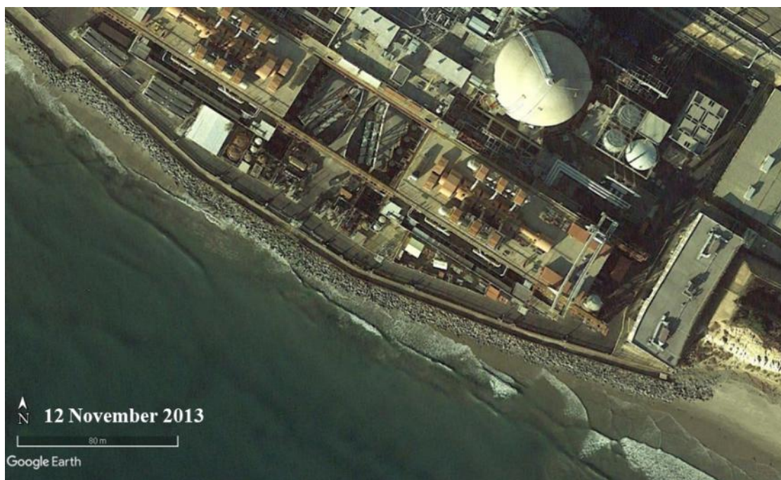
Photo C-12. Photograph showing waves attacking SONGS revetment and refracting towards south at the southern end of SONGS (12 November 2013).
