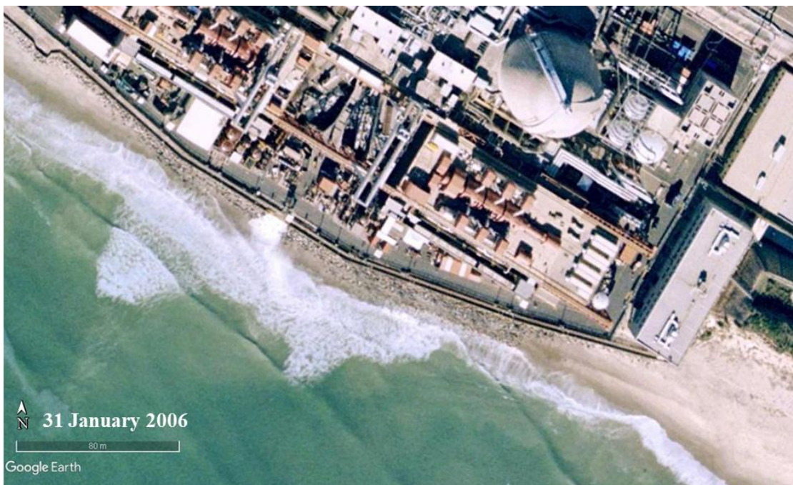
Photo C-8. Photograph showing waves from north swell attacking SONGS revetment and refracting towards south at the southern end of SONGS (31 January 2006).
