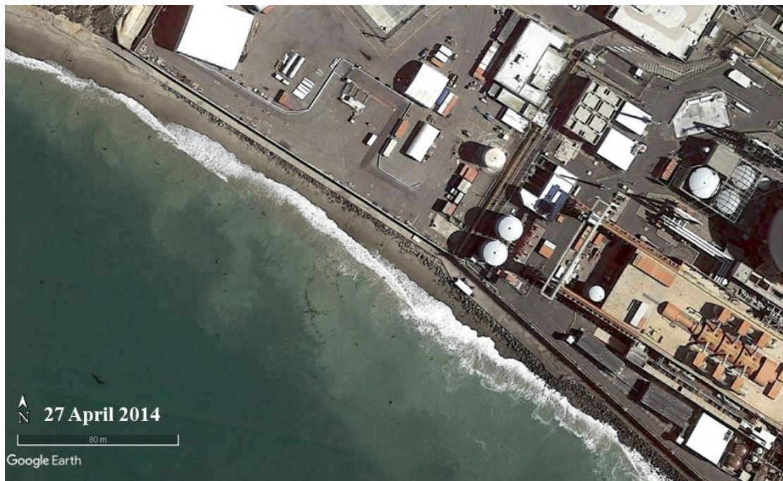
Photo C-13. Photograph showing revetment exposed and fronted by a wide beach at the northern end of SONGS (27 April 2014).
