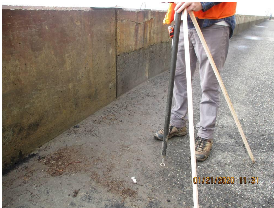
Photo B-20. Benchmark BM10, created on 21 January 2020, is marked by a metal screw and washer and is located on the walkway south of transect S0800'. This benchmark has replaced benchmark 2051613.
