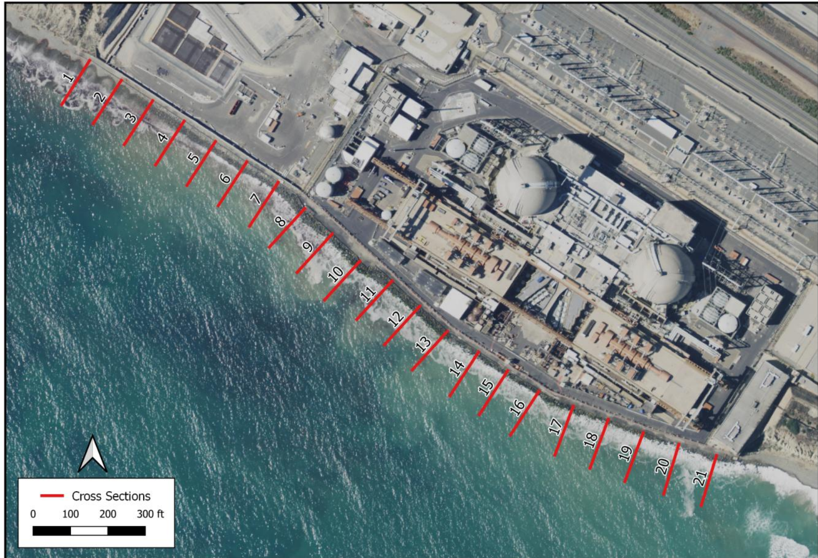
Figure A-1. Locations of 21 transects along the revetment, spaced 100 ft apart.
