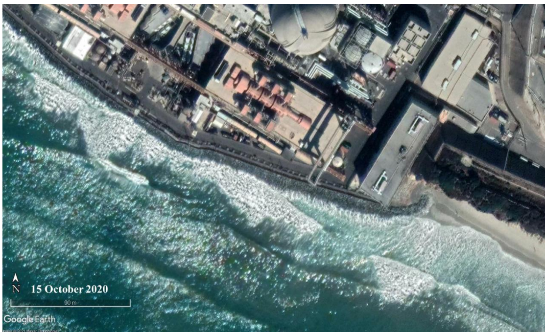
Photo C-20. Photograph showing waves attacking SONGS revetment and refracting towards south at the southern end of SONGS (15 October 2020).
