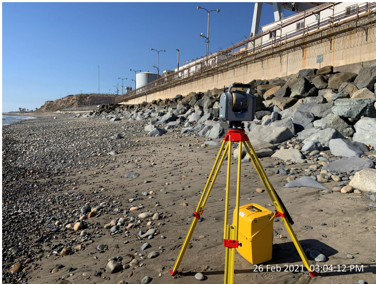
Figure 3-8. Trimble SX10 scanning total station.
