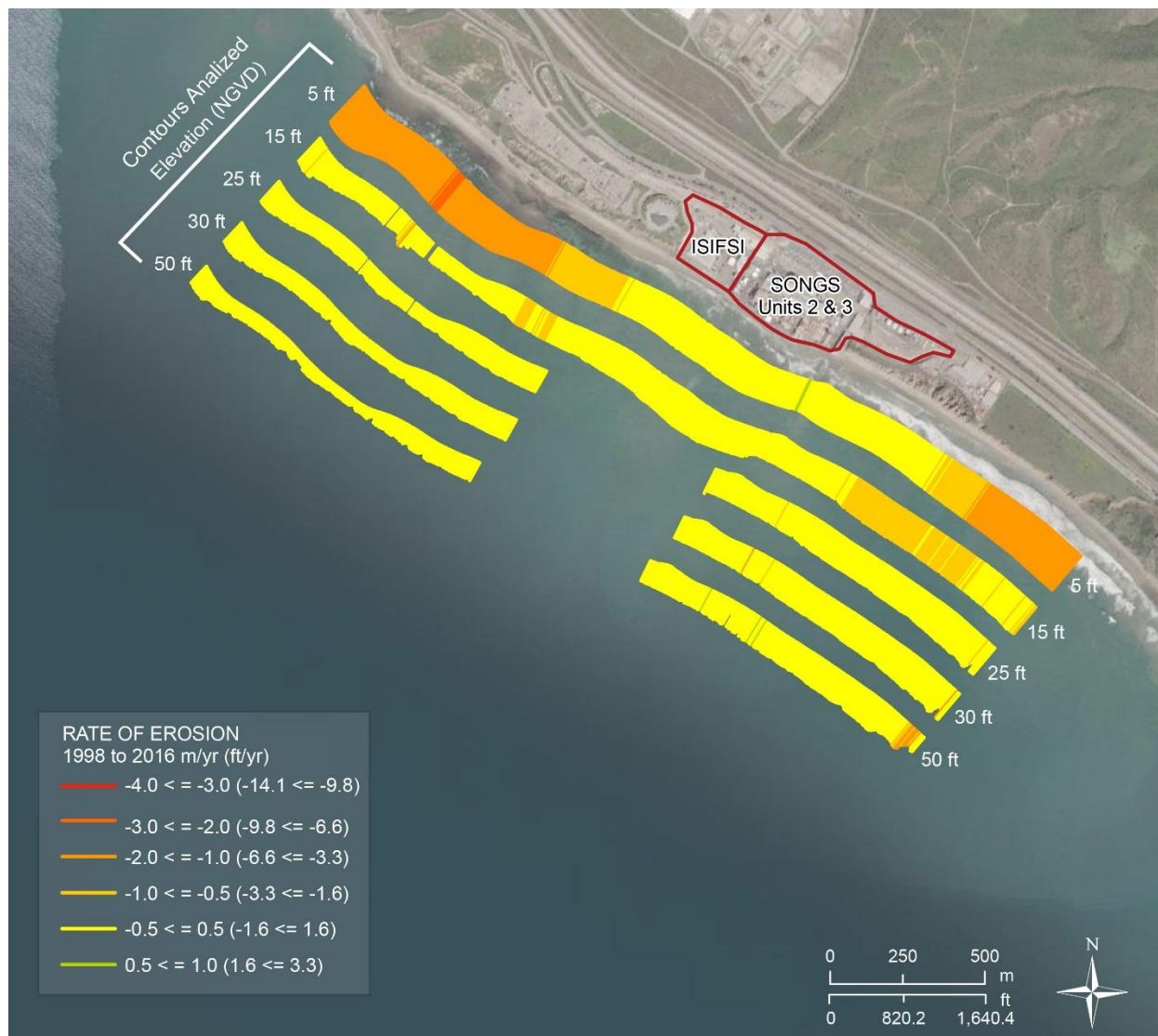
Figure 3-21. Erosion rates for contours at 5, 15, 25, 30, and 50 ft calculated using the DSAS tool from 1998 until 2016.
