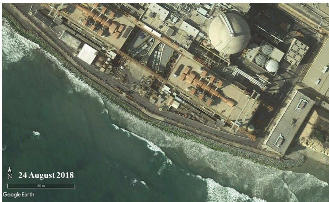
Photo C-18. Photograph showing waves from north swell attacking SONGS revetment and refracting towards south at the southern end of SONGS (24 August 2018).
