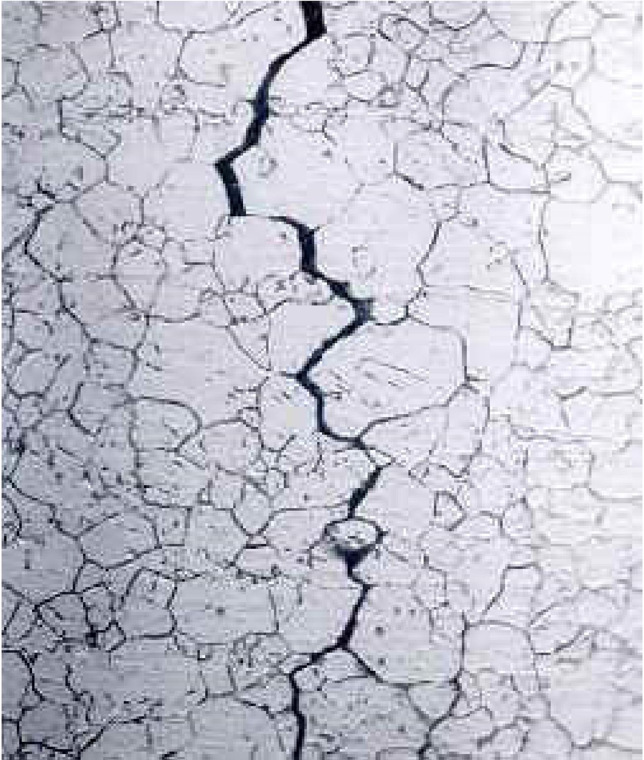
Intergranular Stainless Steel Stress Corrosion Crack with crack following grain boundaries, enlarged X500 <https://www.corrosion-doctors.org/Forms-SCC/scc.htm>
